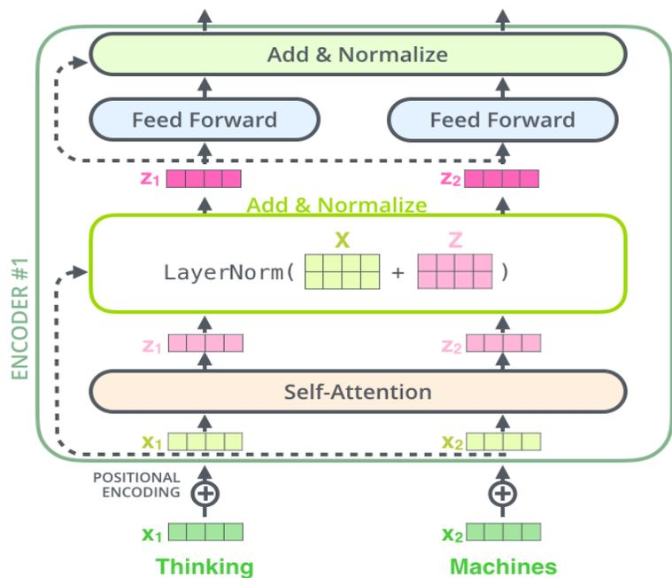
Fig. 1: Encoder Architecture of Transformer
